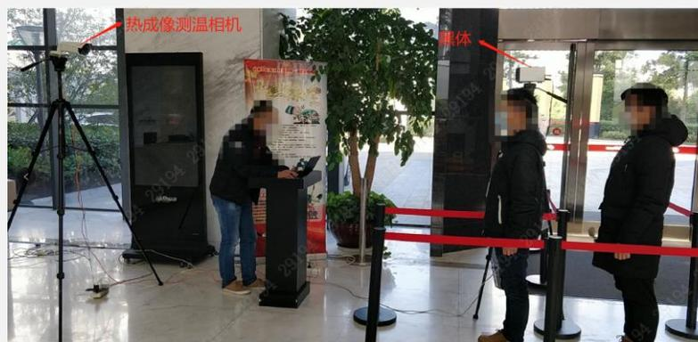
**Convenient deployment:** human body temperature measurement thermal imaging camera + black body + ordinary PC constitutes a small temperature measurement station
